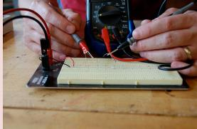
Break the circuit somewhere and then let the multimeter complete it. The current will travel through the meter.
